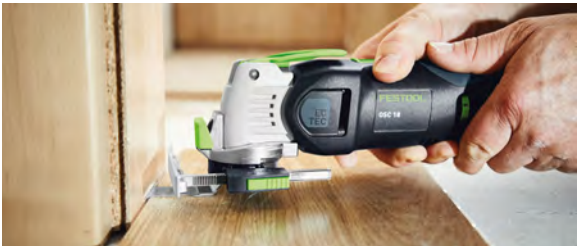
Depth stop Designed for maximum precision, the depth stop lets you set and control the depth of your cut at multiple angles.
