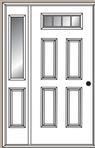
Single Prehung with Sidelite on the Hinge Side
